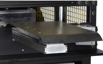
Weldlogic engineers have designed a compact 12 Ton press with hardened tooling to form the ideal lead/lag edges.
